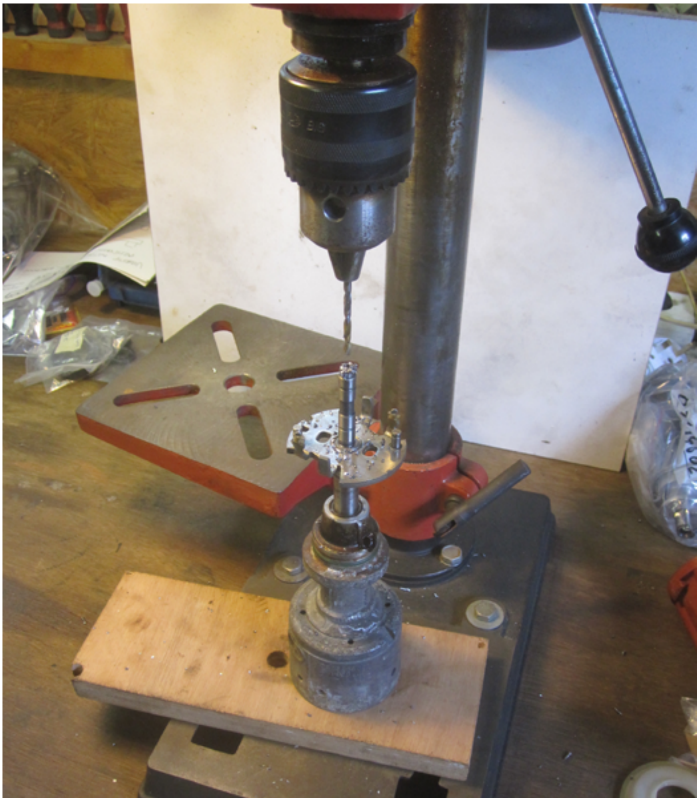
Drilling a hole in the shaft using the VAG distributor body as a jig.
