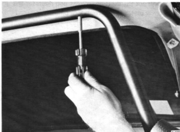
REMOVAL OF SCREWS FOR REAR WINDOW
