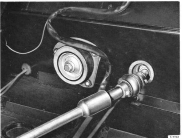
FITTING THE LIMITING WASHER
