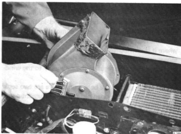
REMOVAL OF FAN CASING
