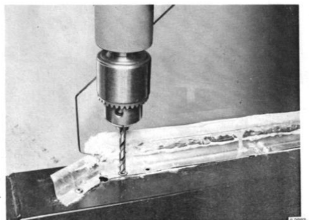
REMOVAL OF POP RIVETS FROM SEALING STRIP, MODEL 1970
