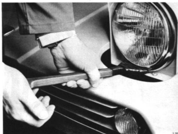
INSTALLING THE HEADLIGHT INSERT
