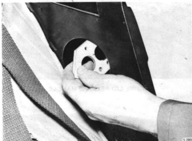
FITTING THE STRIKER PLATE AND RETAINING PLATE
