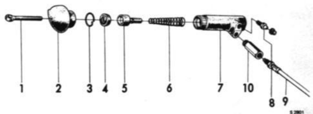
SLAVE CYLINDER, DISASSEMBLED
