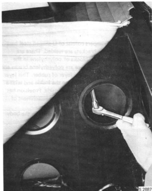
REMOVAL OF ROLL-OVER BAR RETAINING SCREWS
