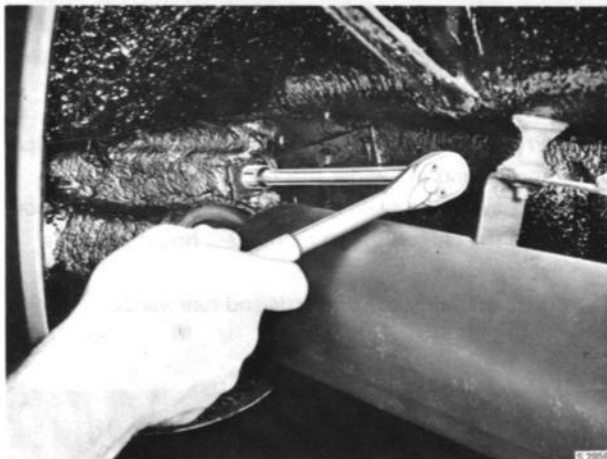
REMOVAL OF NUTS ABOVE THE REAR SILENCER
