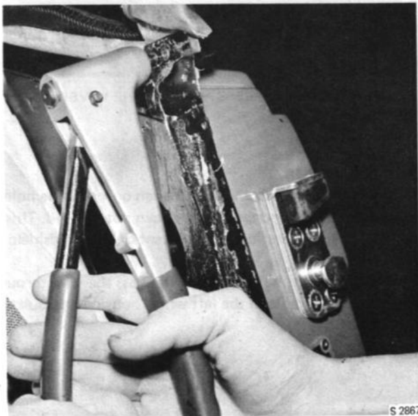
RIVETING WITH A POP RIVET TOOL
