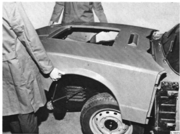
REMOVAL OF HOOD
