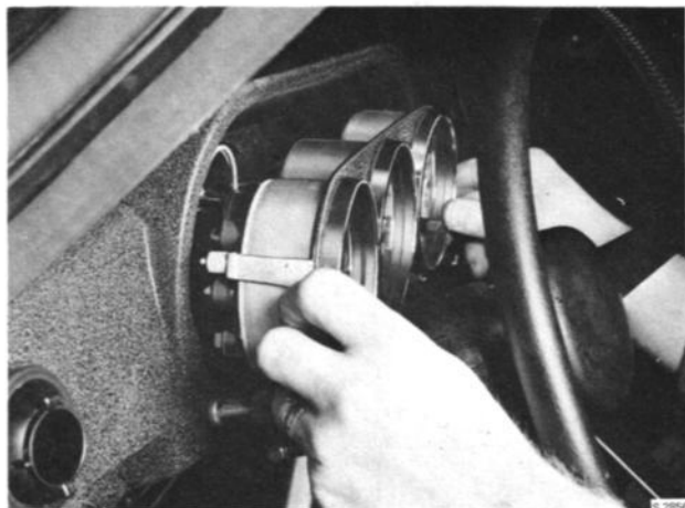
REMOVAL OF INSTRUMENT INSERT
