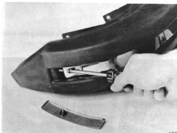
MOUNTING THE BRACING STRIP
