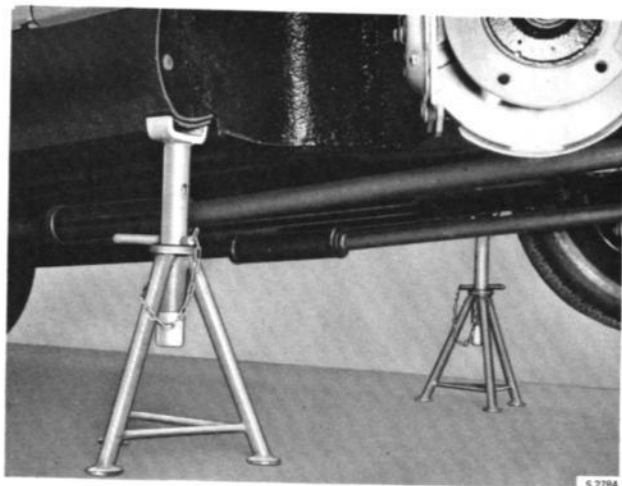
SUPPORTING THE FRONT END ON TRESTLES
