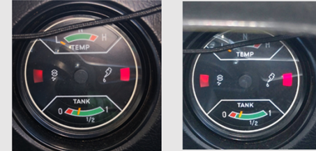
Original Gauge (Left) at 13 litre remaining vs. New Gauge
